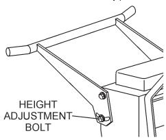
Figure 35. Handle Bar Adjustment Bolts
